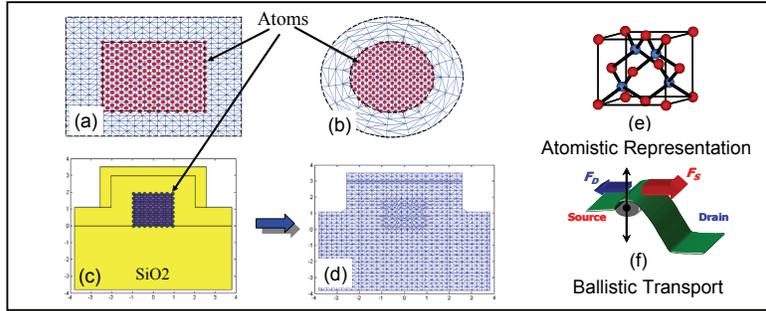
**Figure 1:** The 2D cross sections of the devices treated. The finite element mesh and the atomic positions (dots) are indicated. (a) Rectangular, (b) Cylindrical, (c) The tri-gate device structure, (d) The mesh for the tri-gate structure. (e) The zincblende lattice configuration used for the atomistic description of the device. (f) The semi-classical ballistic model used to calculate device characteristics.
