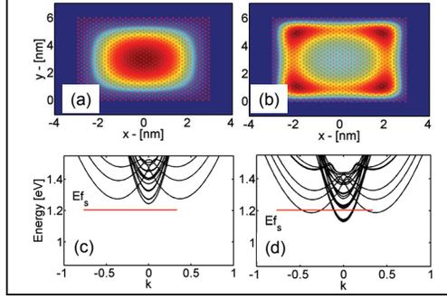
**Figure 3:** Device features for a 6nm rectangular wire. (a-b) The 2D cross section showing the charge distribution under low and high gate biases, respectively. The dots indicate the underlying atomic positions. (c-d) The corresponding  $E(k)$  plots for the cases (a-b).  $E_f^s$  is the source Fermi level.
