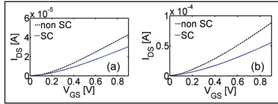
**Figure 4:** The  $I_D$ - $V_G$  characteristics calculated using the empty (non-SC)  $E(k)$  diagram and using the charge filled (SC)  $E(k)$  diagram for the 3nm and 6nm rectangular nanowires. (a) The 3nm device. (b) The 6nm device.
