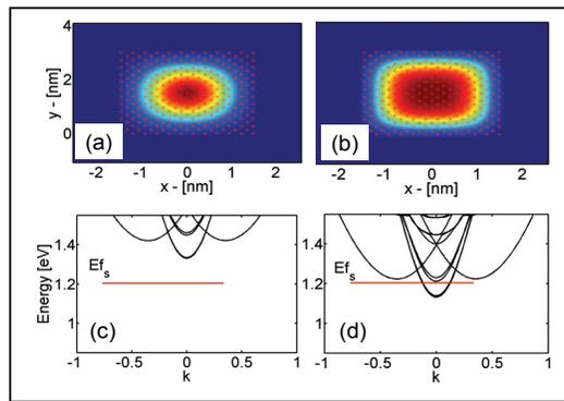
**Figure 2:** Device features for a 3nm rectangular wire. (a-b) The 2D cross section showing the charge distribution under low and high gate biases, respectively. The dots indicate the underlying atomic positions. (c-d)  $E(k)$  plots for the cases (a-b).  $E_f^s$  is the source Fermi level.
