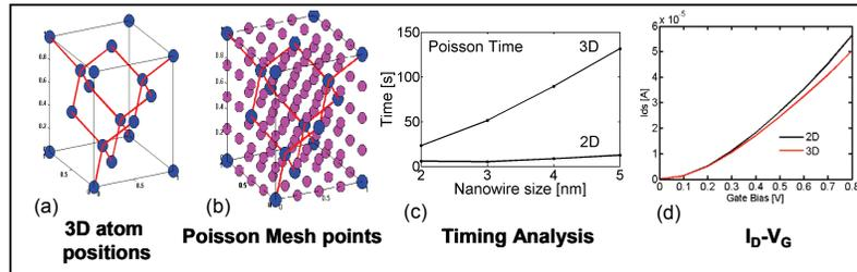
**Figure 5:** (a) The position of the atoms in the zincblende lattice. (b) 3D mesh nodes for the equivalent 2D Poisson. (c) Time comparison between a full 3-D atomistic lattice and a quasi 2-D solution. (d)  $I_D$ - $V_G$  characteristics computed for quasi 2-D and full 3-D Poisson solution.
