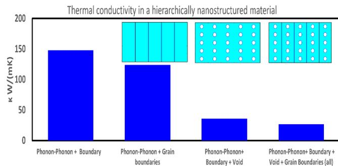
**Figure 1b.:** Thermal conductivity reduction for a typical hierarchically nanostructured material.
