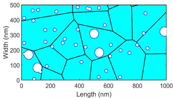
**Figure 1a.:** Geometry of simulation domain including defects, voids and grain boundaries.
